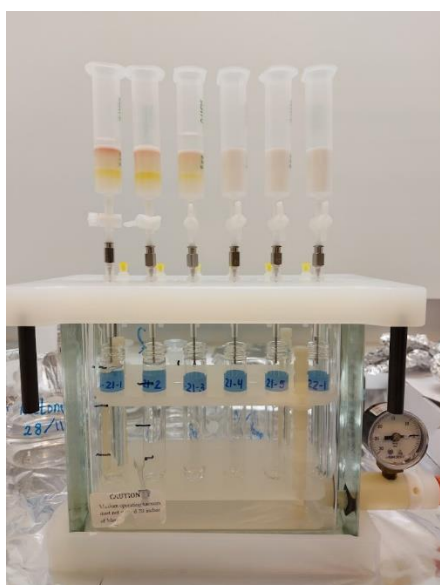
Figure 3: The assembled station for the EZ-POP clean up procedure. Samples have been added to the three cartridges on the left.
